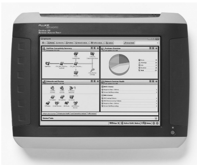
Figure 3.5 OptiView XG network tablet. (Photo provided by Fluke Networks.)
